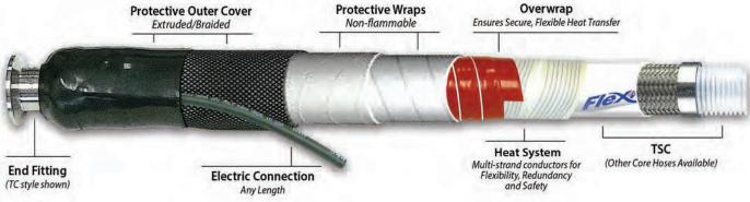
**EHH** is custom manufactured for a variety of applications to keep product flowing. Compared to single conductor heating elements, the **EHH** provides optimal heat transfer to a large (95%) surface area. Individual strand conductors are fixed in place and insulated with flexible, high-temperature fiber. The "Overwrap" layer of silicone rubber secures the conductors and provides a flexible cushion.
