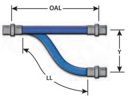
**Note:** Where offset motion "Y" occurs on both sides of hose centerline, the hose live length should be based on total travel, or 2Y. The modified calculation will be:
